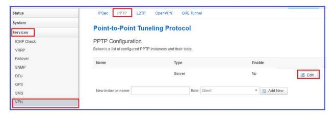
4. Enable PPTP and use a different local subnet for PPTP connection. If the router Lan IP address is the default 192.168.1.1, configure the local IP on PPTP as 192.168.0.1 as shown below. Add username and password.
