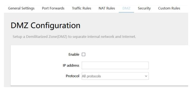
In computer networking, DMZ is a firewall configuration for securing local area networks (LANs).
