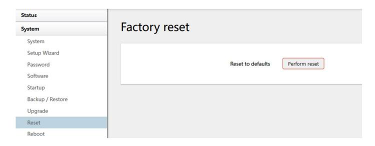
This button resets all configurations to factory default. After clicking the button "Perform reset", a message will appear prompting you to confirm. By clicking "OK", the router will reset to factory default and the system will restart.
