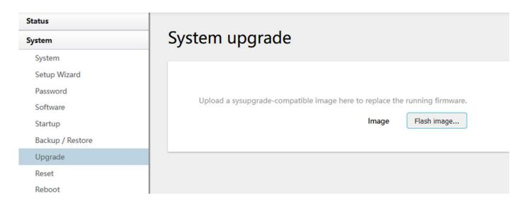
Upload a system compatible firmware to replace the current firmware. Click the button "Flash image" and select compatible firmware, then click the button "Upload". The default value for "Keep settings" is checked, which means the existing configuration will be kept after the system upgrade, otherwise the router will be reset to factory settings. We recommend un-checking "Keep settings" to prevent conflicting parameters after the firmware upgrade.
