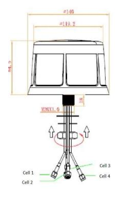
The ANT-LPA-4x4 antenna is IP67 rated, which allows protection against dust and water penetration. It can be mounted externally on a vehicle or on any flat surface such as a kiosk or an ATM machine. The screw-mount kit offers anti-vandal security for peace of mind. It is the perfect solution for M2M applications such as telematics, transportation, and remote monitoring applications.
